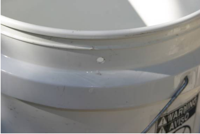
Figure 7. One of two holes to run tubes into bucket
